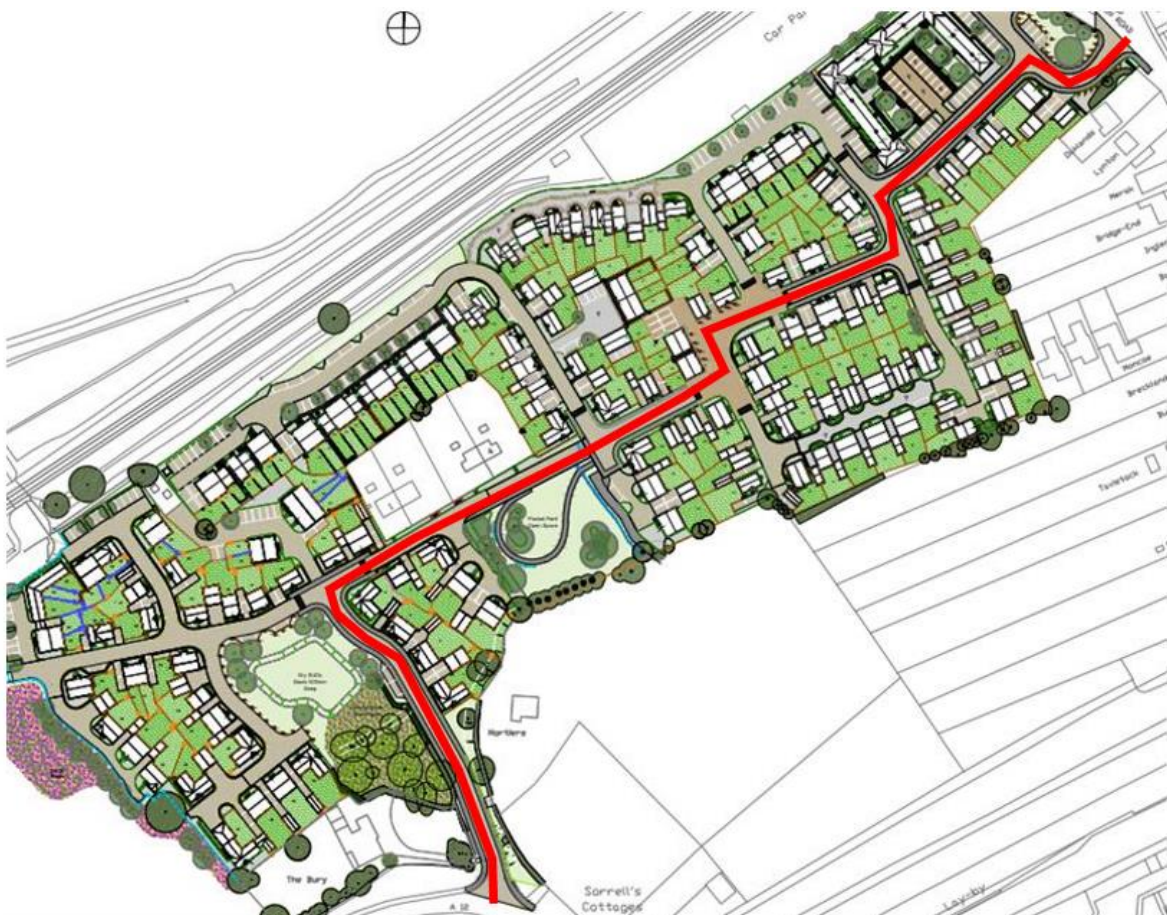
Plate 5.10 Temporary through route
